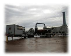
PSI has teamed with Tricilacom Technology Development to provide low temperature thermal desorption services for the remediation of PCB's, pesticides, solvents, coal tar, drilling mud's, dioxins, organic chemicals, mercury and other types of soils, for wastes generated at customer facilities, or for central treatment, storage and disposal facilities.
